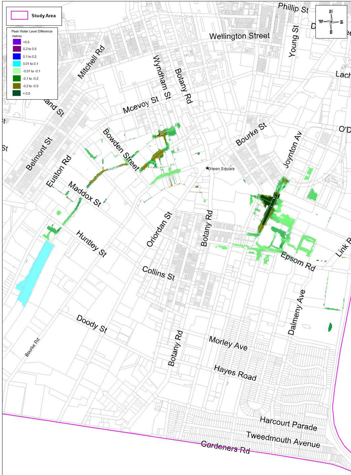
Figure D14 100 Year ARI Peak Water Level Difference for FM9 Less Existing
